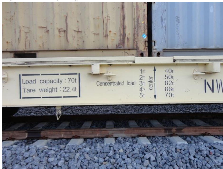
Figure 33: Capacity Label of a 40' Container Rail Car
